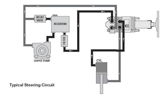
Hydro Boost Install Diagram For Direct
